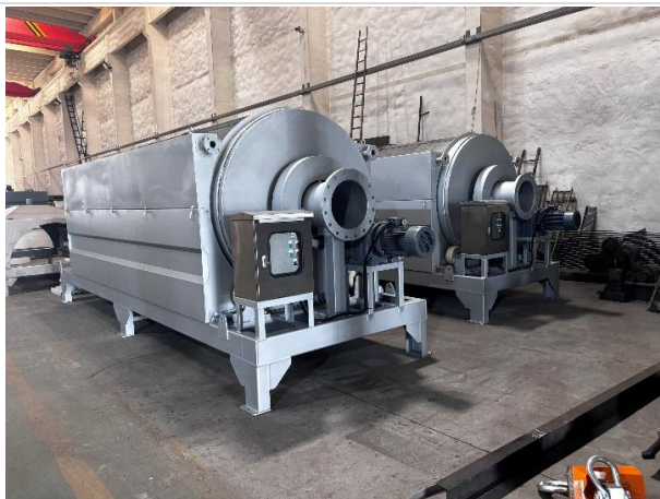
Fig 1 Rotary Drum Screen (JXN-1700X4500)
