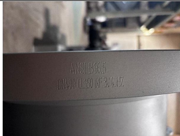
INLET FLANGE DN400 CL150 304
